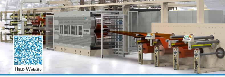
Isobaric Double belt presses (DBP) from HELD are the ideal production systems for the continuous production of roll, sheet and plate materials when using the through-feed method. Various processes, such as continuous laminating, compacting, consolidation, smoothing allow different materials to be processed, like films, fabrics, mats of fibers, granulates or powders. The materials run through the press between two endless steel belts, in single or multiple layers.
