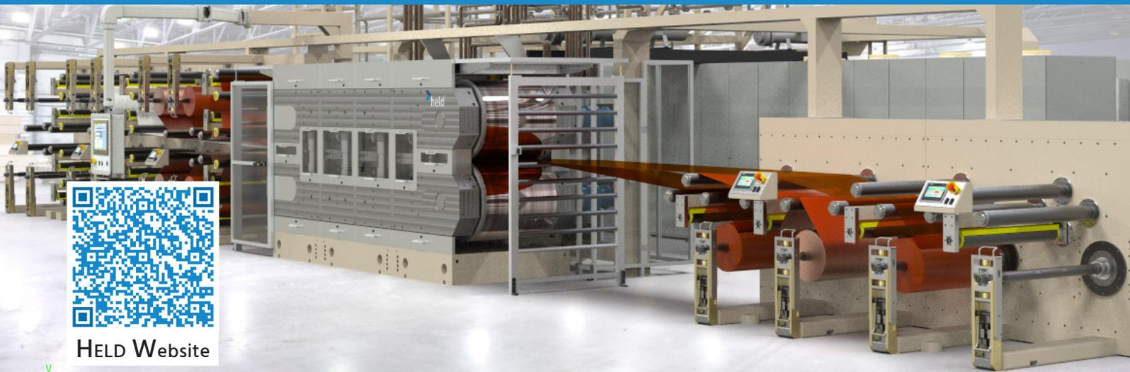
Isobaric Double belt presses (DBP) from HELD are the ideal production systems for the continuous production of roll, sheet and plate materials when using the through-feed method. Various processes, such as continuous laminating, compacting, consolidation, smoothing allow different materials to be processed, like films, fabrics, mats of fibers, granulates or powders.
